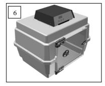
4.5 Fit the M4 x 30mm cap-headed screws, star washers and dome nuts into each set of holes around the edge of the cabinet. Tighten enough to prevent them spinning. This creates an air tight seal around the cabinet.
