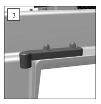
4.4 Place the door in the lower hinge and close the latch. Lower the top cabinet down onto the other parts.
