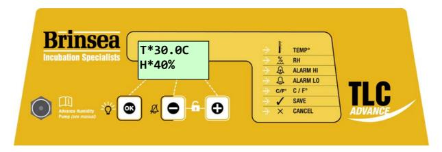
The TLC Advance control system utilises highly accurate, individually calibrated sensors for temperature and humidity. Be cautious of low cost analogue or digital thermometers and hygrometers when comparing them with the brooder display readings.
