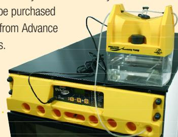
Humidity Pump Module connected
