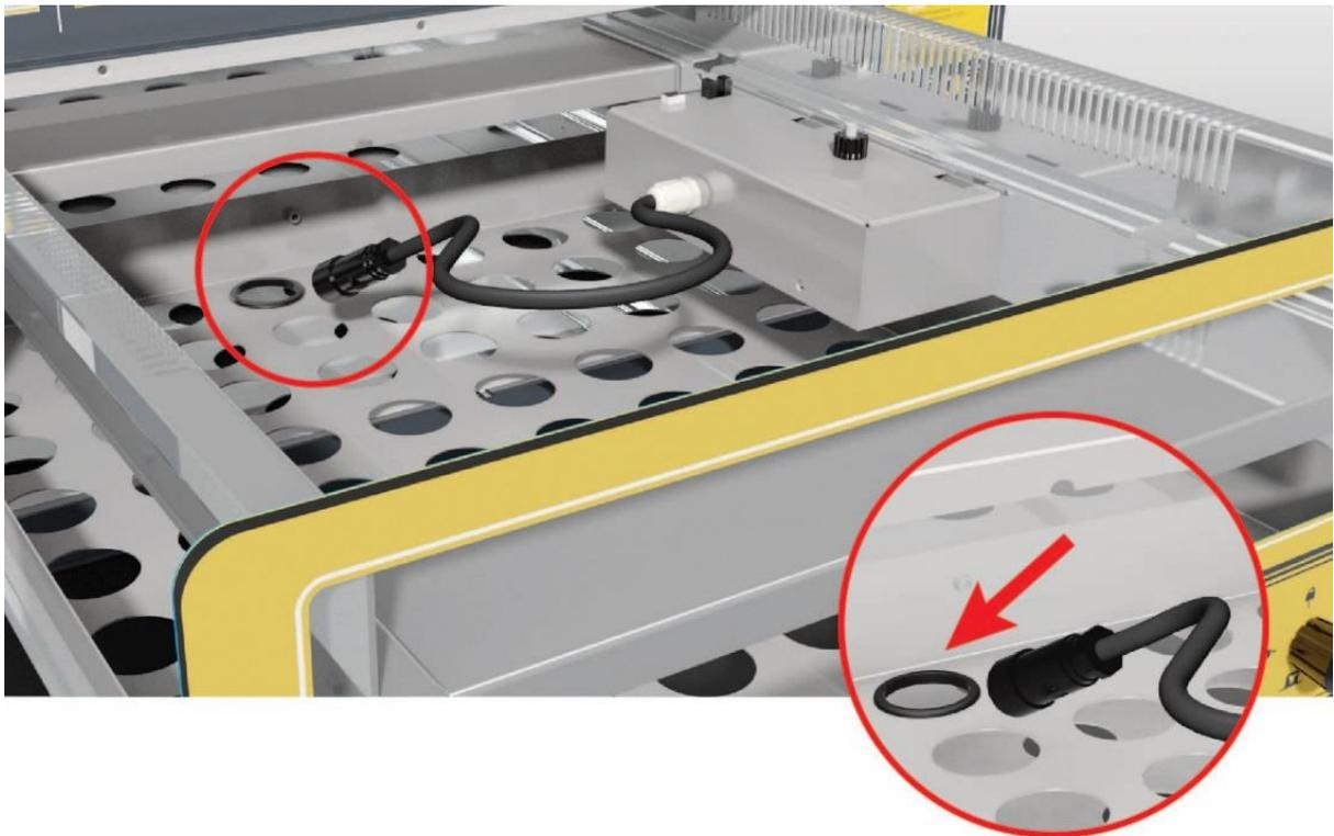
Gently pull the cable through into a loop ready to plug into the incubator socket.
