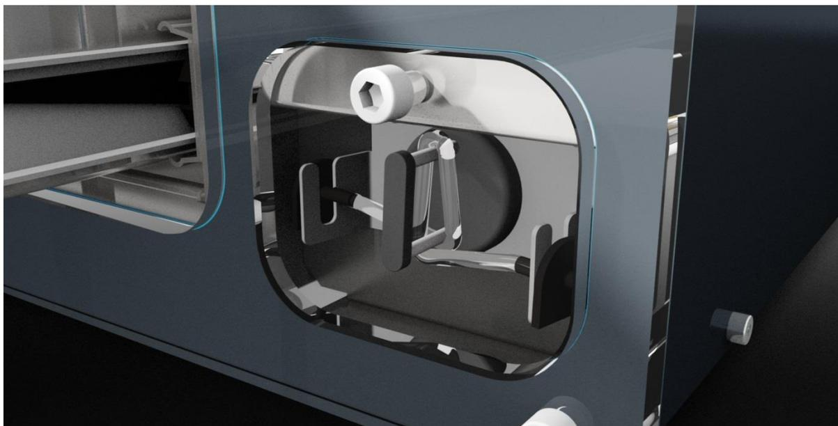
The tube that is held around the pump capstan is of precise length to ensure it is correctly “pinched” where it rolls on the capstan pins. It will wear out during extended use and should be replaced periodically with a new length of tube 110mm long. This length is shown below for reference:
